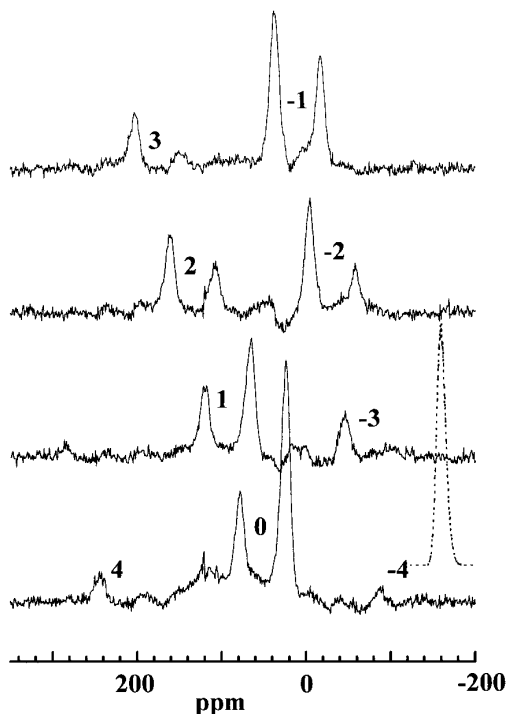
FIG. 8. ^{13}\text{C} MAS NMR spectrum of \text{Yb}(\text{C}_2\text{D}_5\text{SO}_4)_3 \cdot 9\text{H}_2\text{O} at the ^{13}\text{C} resonance frequency of 75.56 MHz. The spectrum was recorded by a five-pulse PASS sequence (25) without ^1\text{H} decoupling. The spinning frequency was 3.1 kHz; 1024 transients are accumulated for each experiment with a recycle delay of 10 s. The four subspectra show well-resolved sidebands separated by the four multiples of the spinning frequency. The numbers on the spectra show the orders of the spinning sidebands. The dotted line is a spectrum calculated by taking account of the polycrystalline effect. The line position is shifted for appearance.
